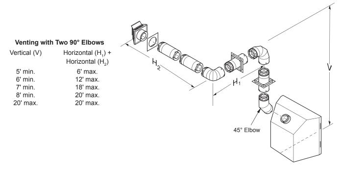
Figure 18 - Horizontal Termination Configuration for Venting Using Two 90° Elbows with Termination at 90° with Fireplace
